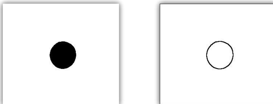
Figure 3.3: Thresholded image before and after edge detection with a 2D Sobel convolution filter.
